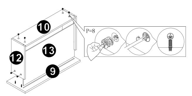
STEP 13-3:Fix rails (N-2) to panel (11) (12) with screw (V1)
