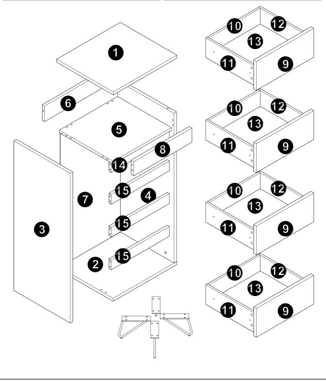
STEP 1: Fix dowel (B) and cam pin (A) to panel (2) (3) (4) (5). B=20
