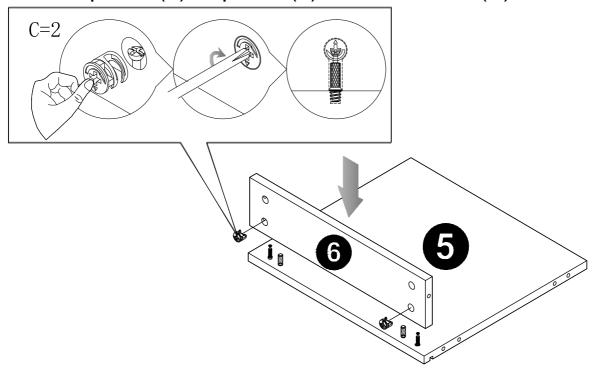
STEP 4:Fix panel (8) to panel (5) with cam lock (C).
